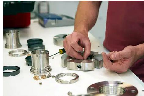
We replace, repair, retrofit and upgrade any mixer seal. Direct drop in replacement seal, with certs. It is single dry running, 316ss, FDA carbon face vs FDA Silicon carbide face with FDA EPDM elastomers. USP VI elastomers and seal faces are available as well as non-squealing design for upgrades.
